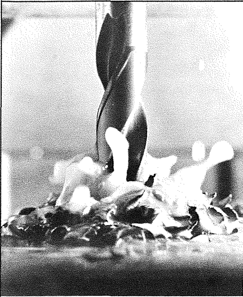
A Jet Pulser assisted drill "digs in" at 500 revolutions per minute.
